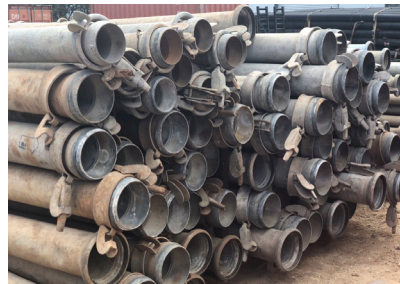
QD Piping, HDPE Piping, Hoses, & Fittings
